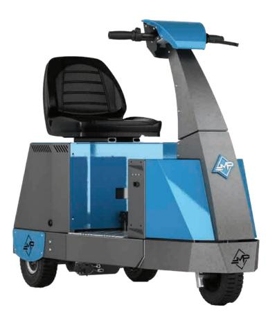
A compact tractor able to easily transport a person and a tow up to 1000 kg in complete safety.
