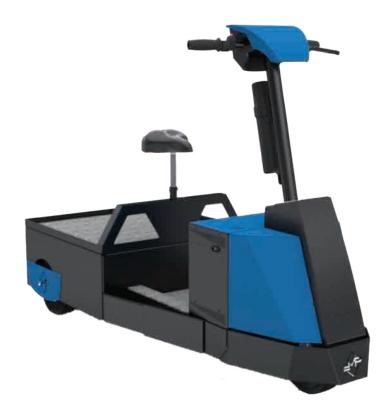
A compact and robust platform particularly suitable for those companies where picking is intensive. The floor where the references are stored is raised, wide and separated from the driving position to increase the safety of the driver and goods.
