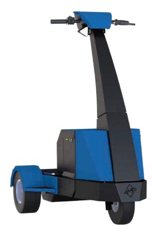
A real electric tractor, to move on large industrial surfaces and transport a person and a tow up to 500 kg safely.
