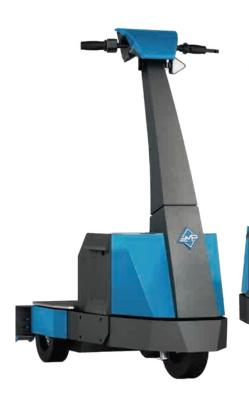
Useful and dynamic electric vehicle developed for repositioning supermarket trolleys.
