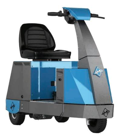
A compact tractor to transport an operator and tow up to 500 kg effectively and safely.
