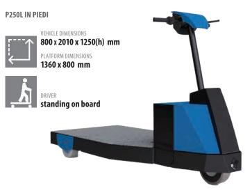
A modern and versatile electricporter for the transport of goods and for the preparation of orders with picking on the ground.
